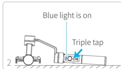
Lay the gimbal on a static flat surface and triple tap the function button. Initialization is successful when the blue light changes from constant on to flashing 3 times periodically, otherwise fail.
