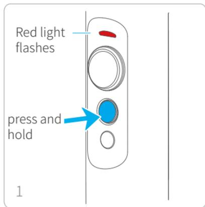
Long press function button and release it until the red light flash, the gimbal enter the standby mode, the blue light will flash 3 times periodically.
