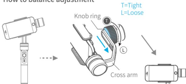
If the smartphone tilted to the left, then loose the knob ring, move the cross arm to the right, try to adjust to the best balance and tight it.
