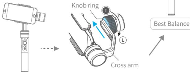
If the smartphone tilted to the right, then loose the knob ring, move the cross arm to the left, try to adjust to the best balance and tight it.
